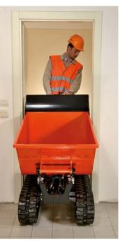
With a minimum overall width of only 758 mm (for all versions) the KC70-4 efficiently transports material through gates and doorways, between houses, buildings and many other narrow spaces. This makes it the perfect mini-dumper for renovations and urban areas.
